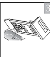
Pull out condensate water
